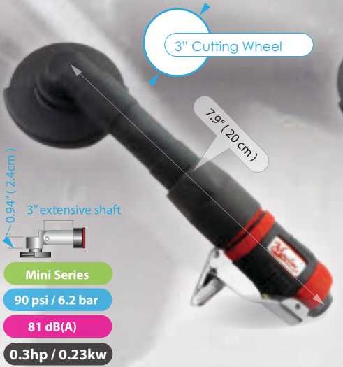
18060 Low Profile Angle Palm Mini Series 3" Extensive Long Neck Shaft 3" Right Angle Cut-off Tool ■ Free Speed: 19000 rpm ■ Optional Muffler MSA-005A
